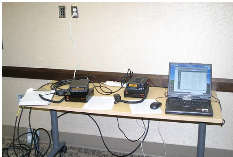
Figure 13: Table set up in Conf. Rm. A with radios and the laptop for packet. Radio to the left is for voice and the radio to the right is for packet.
